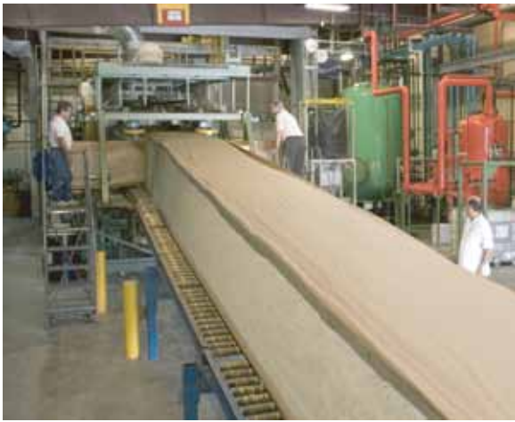
ISO-C1 Polyisocyanurate Bunstock Exiting the Production Tunnel.
