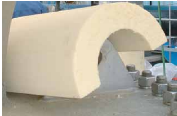
ISO-C1 Fabricated into a Hemi-cylindrical Segment, ready for installation
