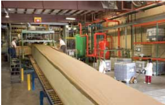
ISO-HT Polyiso Bunstock Exiting Production Tunnel at Dyplast Facilities in Miami
