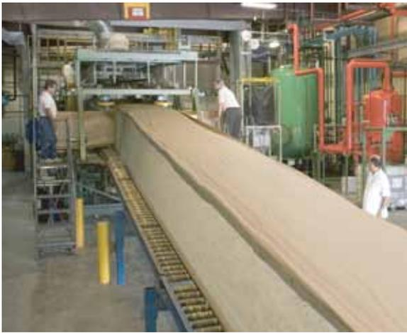
ISO-C1 Polyisocyanurate Bunstock Exiting the Production Tunnel.
