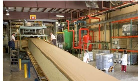
Figure 1: Polyiso exiting the tunnel
